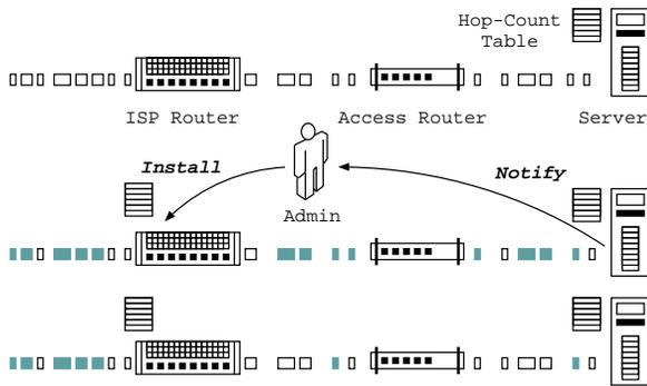
Figure 16: Packet filtering at a router to protect bandwidth.
