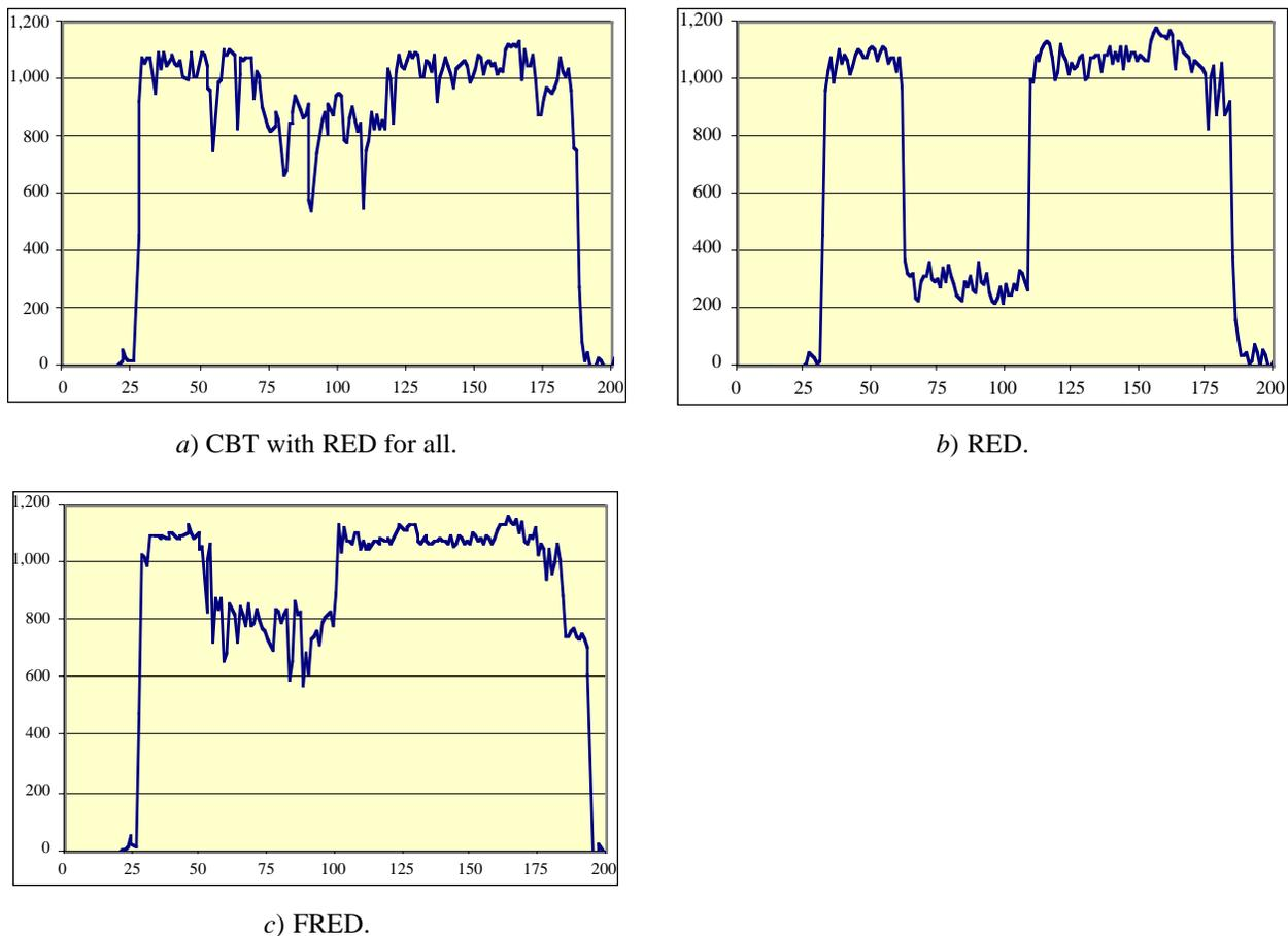
**Figure 5:** Aggregate TCP throughput under “CBT with RED for all,” plain RED, and FRED.
