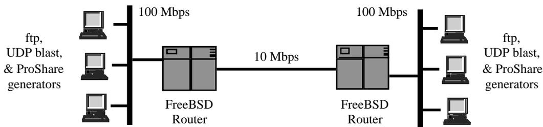
**Figure 4:** Experimental Network Setup
