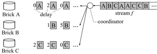
Figure 5: **The improved approach.** Only the aggregate cost of virtual requests is communicated, indicated by the number before each request (assuming unit cost of each request). Broadcasting is avoided yet total service proportional sharing can be achieved.
