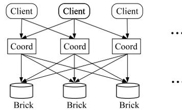
Figure 2: **Data access model of a distributed storage system.** Different clients may have different data layouts spreading across different sets of bricks. However, coordinators know all data layouts and can handle requests from any client.
