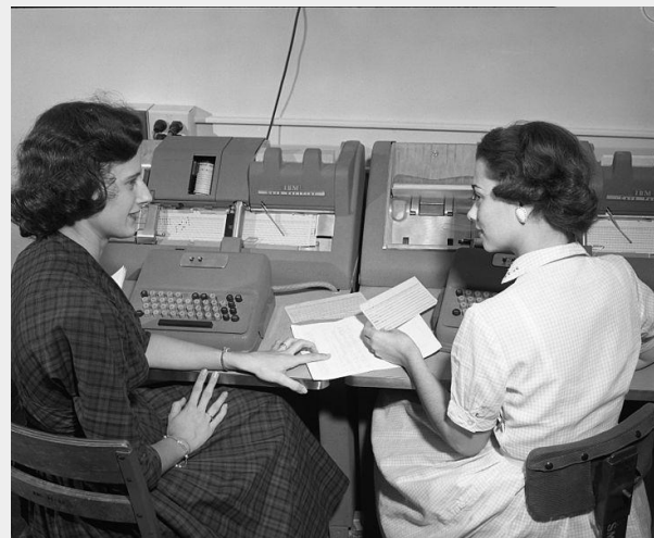
Early example of code review/pair programming; Card Verifier (left) and keypunch (right)
