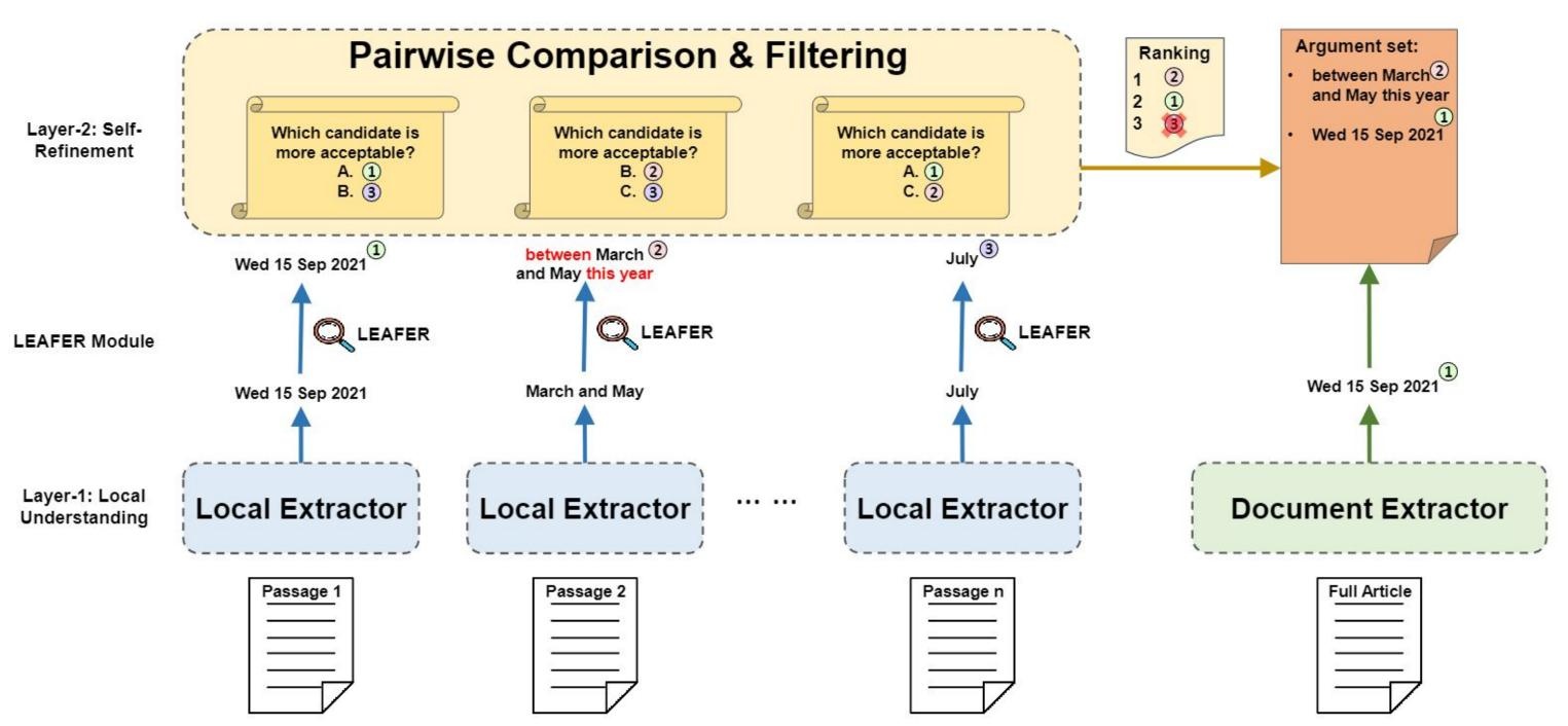
Overall architecture of **ULTRA+**, consisting of **ULTRA** (*left part*) and a document-level extractor (*bottom right*). The underlying model is Flan-UL2.
