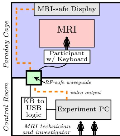
**Figure 4: Illustration of fMRI writing setup. The participant lies in the bore of the fMRI machine, and the keyboard’s cables are connected through an RF- and MRI-safe waveguide. The waveguide connects to the control room, where we attach the keyboard logic to an experiment PC displaying our editing environment. The video output of the experiment PC feeds through the waveguide to connect to an MRI-safe monitor which can be seen by the participant in the MRI bore via mirror projection.**
