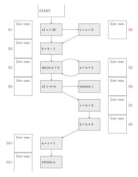
(1 point each) For each basic block **B1** through **B11**, write down the list of variables that are live *right before* the start of the corresponding block in the control flow graph above. Please list only the variable names in lowercase without commas or other spacing (e.g., ab to indicate that a and b are alive before that block.
