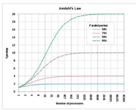
Evolution according to Amdahl's law of the theoretical speedup in latency of the execution of a program in function of the number of processors executing it, for different values of p. The speedup is limited by the serial part of the program. For example, if 95% of the program can be parallelized, the theoretical maximum speedup using parallel computing would be 20 times.
