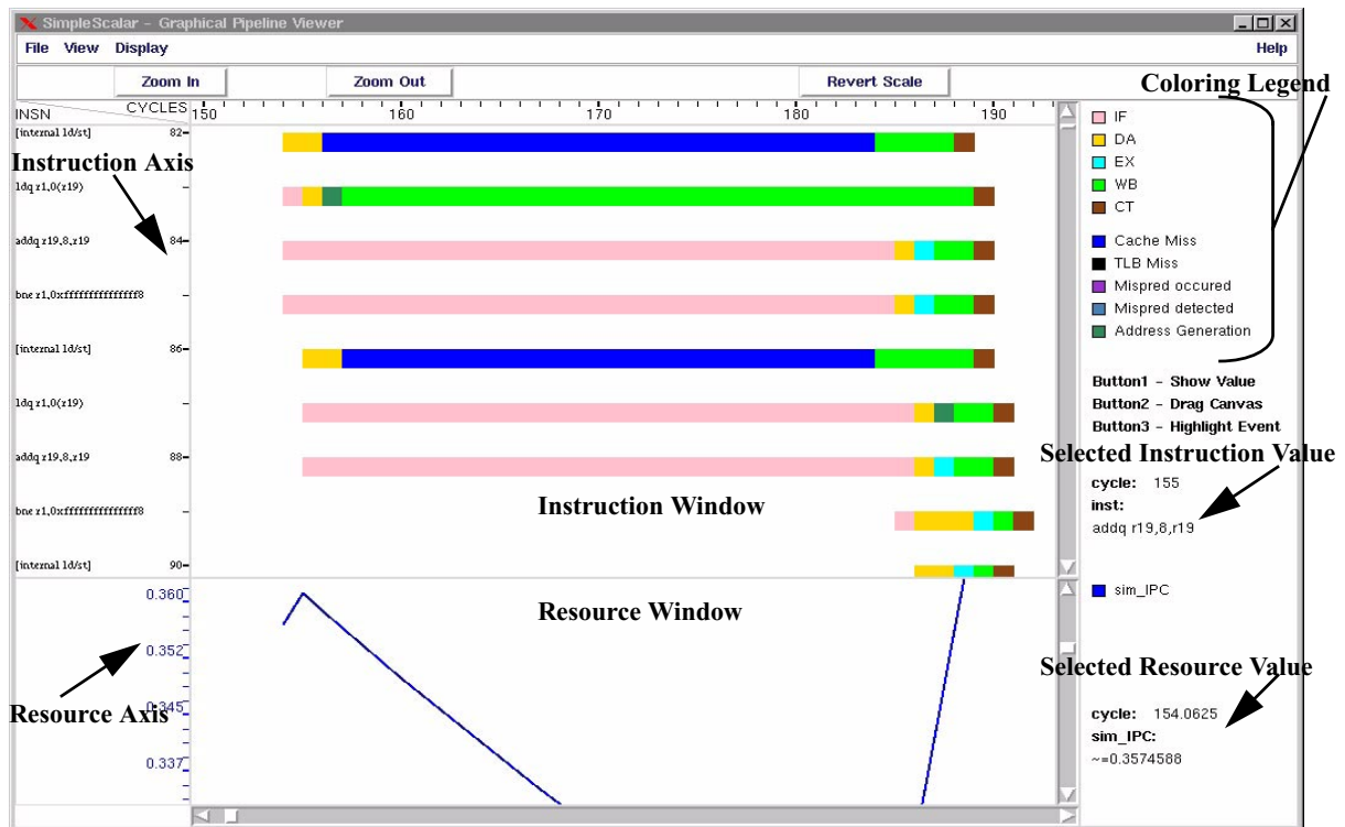
Figure 2 GPV Display Window showing the execution of instructions on a 4-wide Alpha ISA model (note that internal micro-code operations, i.e. internal ld/st, are allowed to finish out of program order)
