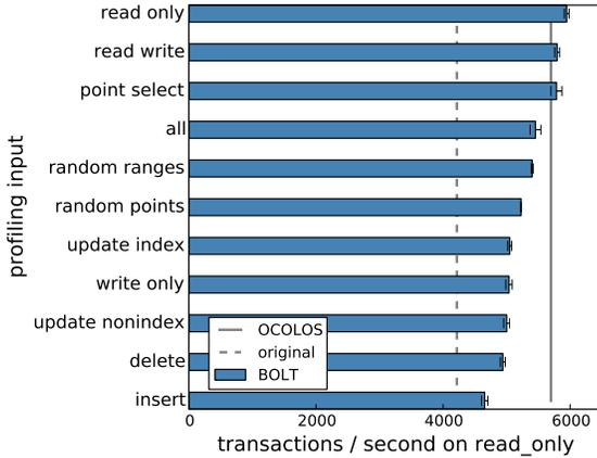
Fig. 3: Performance achieved when running MySQL with the Sysbench `read_only` input, using BOLT to produce a binary from the given profiling input or, with the *all* bar, from profiles of all inputs combined.
