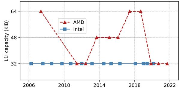
Fig. 1: AMD & Intel per-core L1i capacity over time
