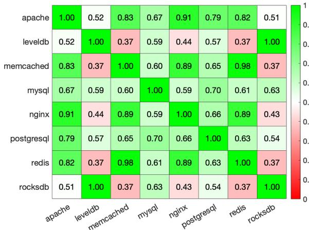
Figure 1: Confusion matrix using cosine similarities for different data center applications based on the Linux kernel’s function execution frequencies: apart from LevelDB and RocksDB, all other applications exhibit close similarity in their kernel function usage.
