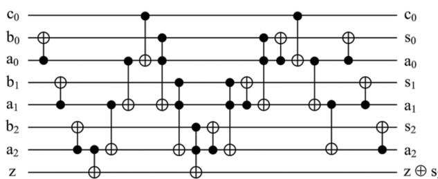
Figure 2 : The proposed 3-bit ripple-carry adder circuit.
