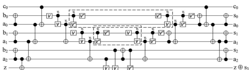
Figure 3 : Quantum equivalent circuit of proposed adder design.
