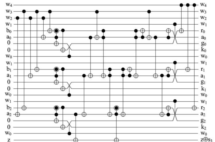
Figure 4 : Proposed design of 3-bit ALU circuit.
