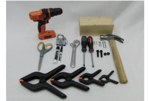
Fig. 3: Tool items in the YCB Object Set: back: power drill, wood block; middle row: scissors, padlock and keys, markers (two sizes), adjustable wrench, phillips and flat screwdrivers, wood screws, nails (two sizes), plastic bolt and nut, hammer; front: spring clamps (four sizes).
