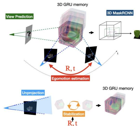
Figure 2. **Geometry-aware Recurrent Neural Networks (GRNNs)** integrate visual information over time in a 3D geometrically-consistent deep feature memory of the visual scene. At each frame, RGB images are *unprojected* into corresponding 3D feature tensors, which are oriented to the coordinate frame of the memory map built thus far (2nd row). A 3D convolutional GRU memory is then updated using the egomotion-stabilized features as input.
