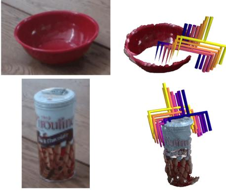
Fig. 7: An example of a grasp refinement process from [41], where the initial grasp is shown in dark blue and the final grasp pose is shown in yellow. ©2019 IEEE)
