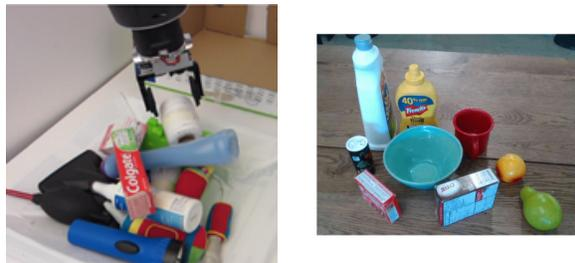
Fig. 13: Examples of cluttered scenes. We differentiate Piled Clutter (left) from Structured clutter (right). Left image is from [38] (©2017 SAGE) and Right image is from [47]. (©2020 IEEE)
