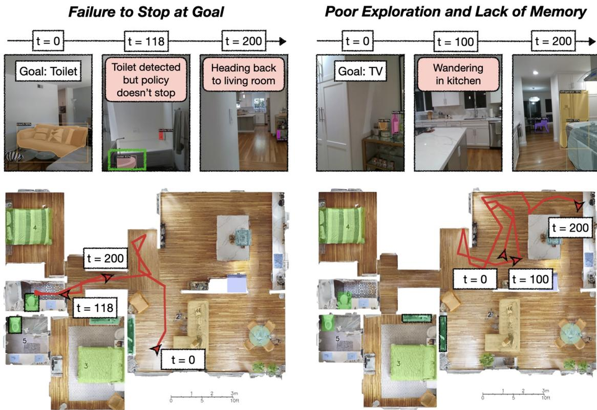
**Fig. S3. Failure modes of end-to-end learning.** (A) The end-to-end policy detects the toilet goal but fails to stop and heads back towards the living room. (B) The end-to-end policy fails to explore effectively, revisiting the same locations in the kitchen while looking for a TV.
