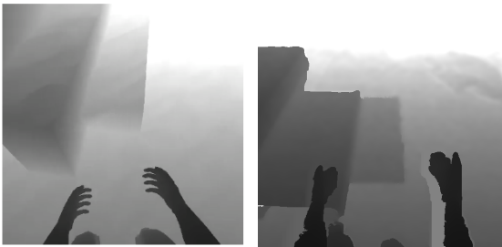
Fig. 9: Sim-to-real camera mapping . Left: simulation rendering. Right: real image captured by the G1 head-mounted camera.
