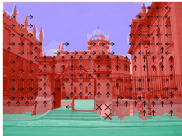
Figure 1: Geometric context from a single image: ground (green), sky (blue), vertical regions (red) subdivided into planar orientations (arrows) and non-planar solid ('x') and porous ('o').
