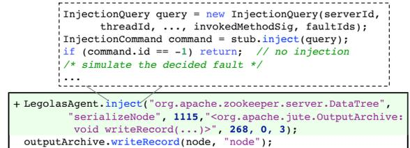
Figure 4: Injection hook instrumented for code in Figure 1.
