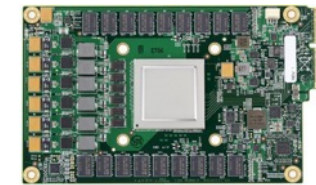
Tensor Processing Unit
