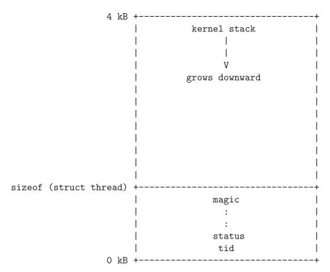
This has two consequences. First, struct thread must not be allowed to grow too big. If it does, then there will not be enough room for the kernel stack. The base struct thread is only a few bytes in size. It probably should stay well under 1 kB.
