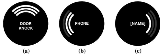
Figure 3. The smartwatch display shows the *direction*, *loudness*, and *identity* of sounds, such as: (a) a loud door knock in front of the wearer, (b) a moderate phone ringing to the left, and (c) a quiet name called to the right.
