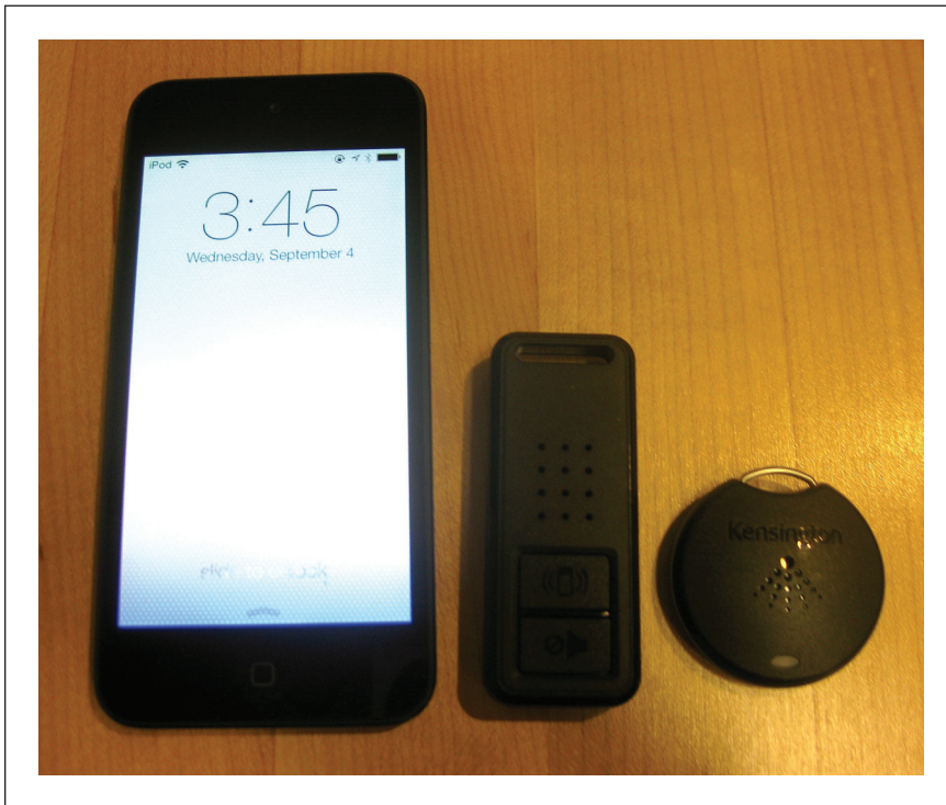
Figure 5. A proximity solution: (a) a smartphone app with (b) a locator fob and (c) the Kensington Proximo LE tag.
