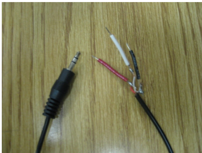
Figure 13: Modified headphone cable for ECG signal
