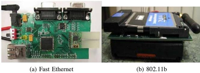
Fig. 7. Base Stations for ECG monitoring System
