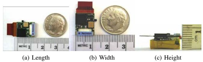
Fig. 5. Eco Dimensions:  $13(L) \times 11(W) \times 7(H)$  mm
