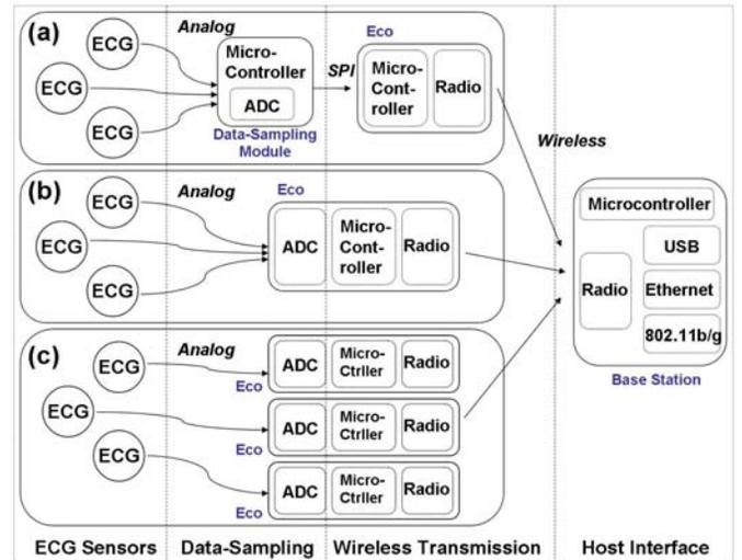
Fig. 2. System Architecture of ECG Monitoring System
