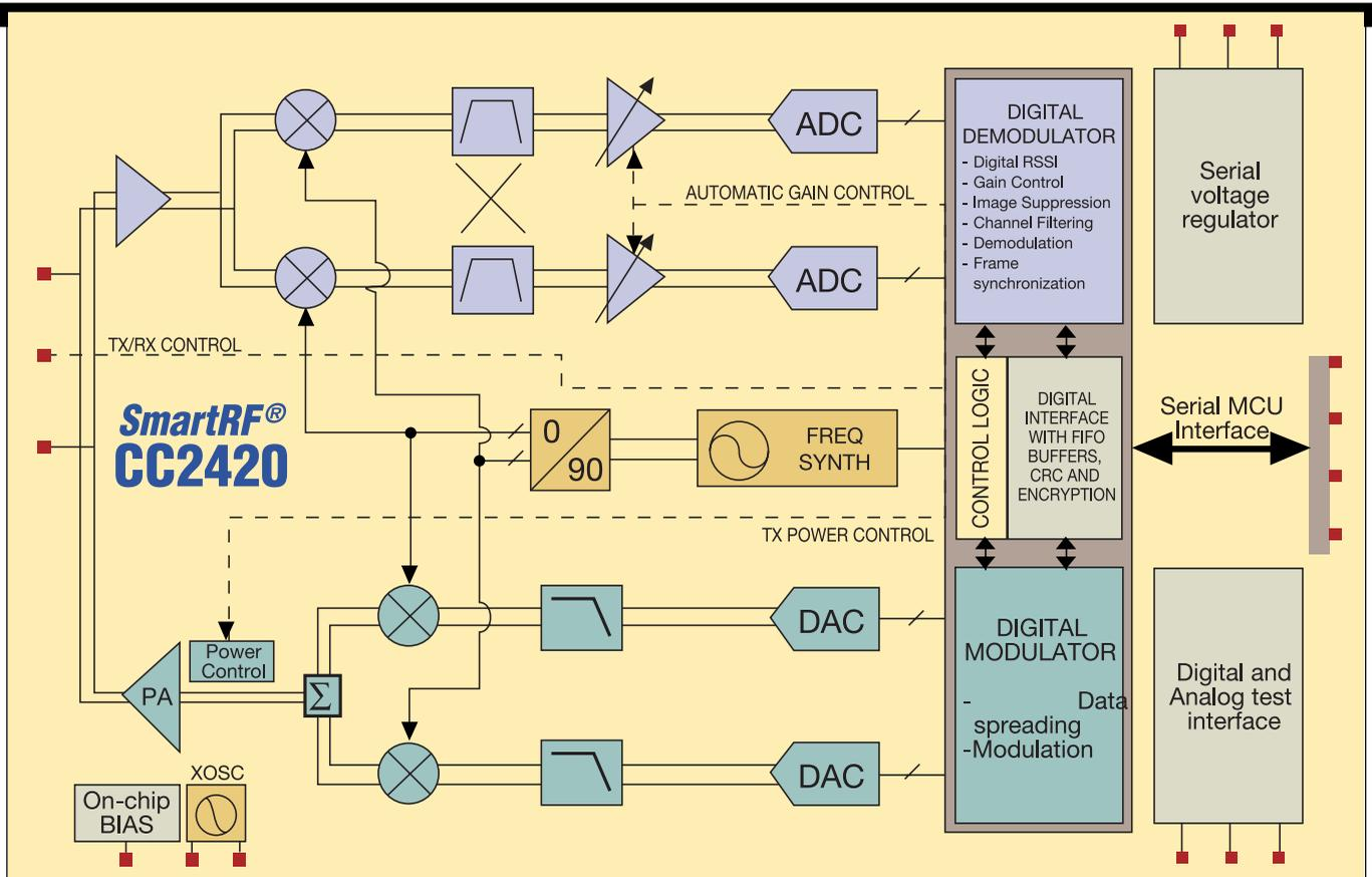
Figure 6. IEEE 802.15.4-compliant and ZigBee-ready CC2420 radio transceiver.
