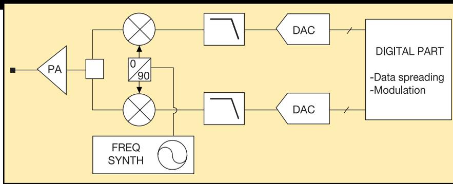
Figure 4. I/Q-modulation transmitter topology.
