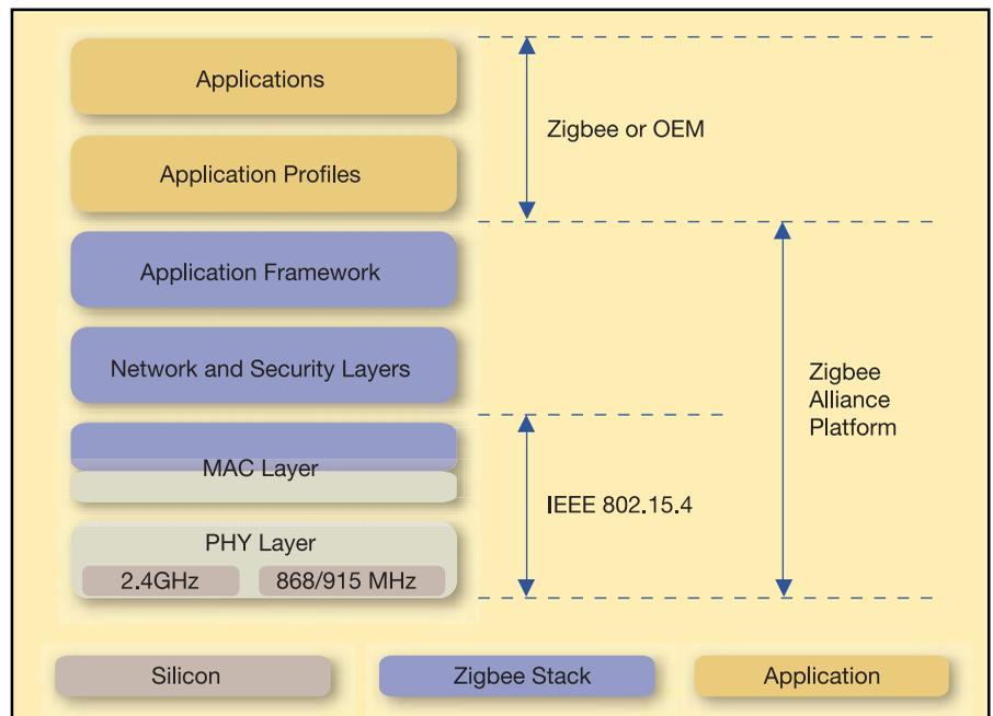
Figure 1. IEEE 802.15.4 and ZigBee working model.
