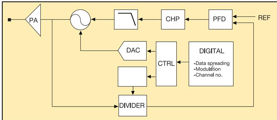
Figure 5. Two-point modulation transmitter topology.
