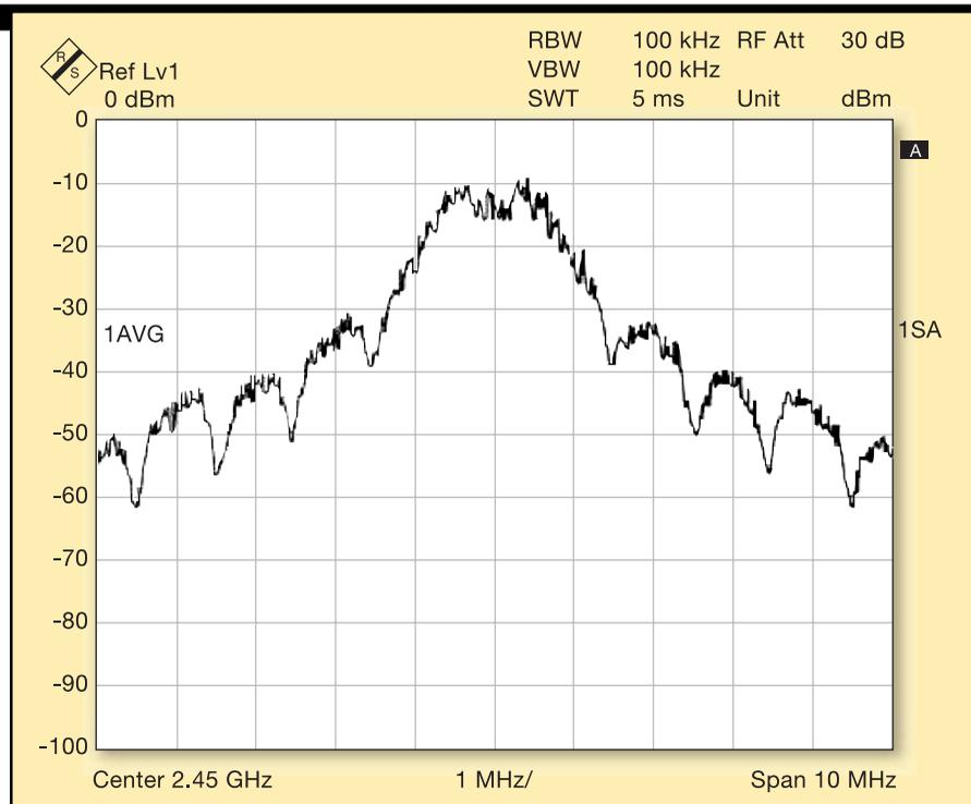
Figure 7. Output spectrum of the CC2420 transmitter.
