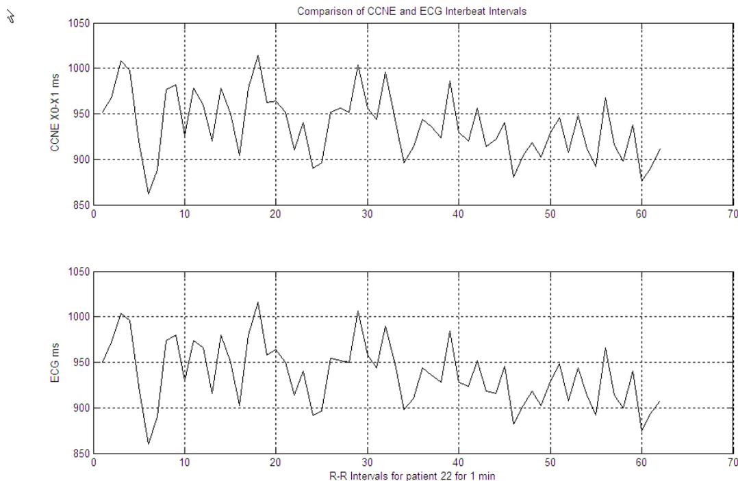
**Figure 6:** Comparison of R-R Interbeat Intervals of CCNE and ECG Electrodes for 1 min.
