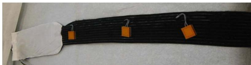
**Figure 3:** Arrangement of Sensors on Strap
