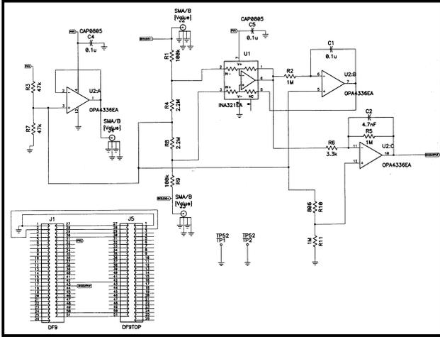
Fig. 2. Schematic of the *EKG on Mica2* circuitry
