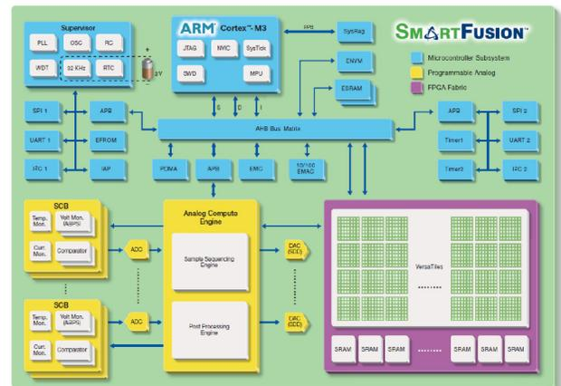
AHB-Lite supports single bus master and provides high-bandwidth operation
