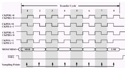
Timing Diagram – Showing Clock polarities and phases
