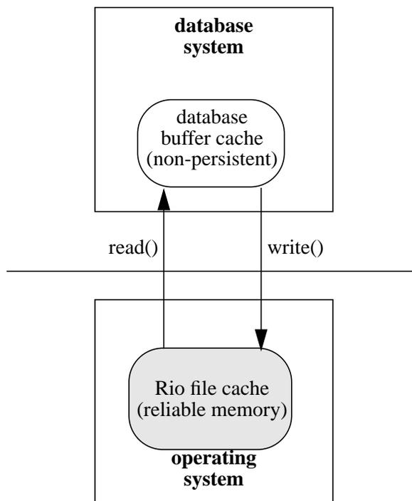
**Figure 3: I/O Interface to Reliable Memory.** This design hides the reliable memory under the file system interface. The database uses `read()` and `write()` system calls to write data to the reliable memory. This design uses a traditional, non-persistent database buffer cache and thus requires change to the database. Because the interface to stable storage has not changed, this design is as safe as a standard database system from database crashes.
