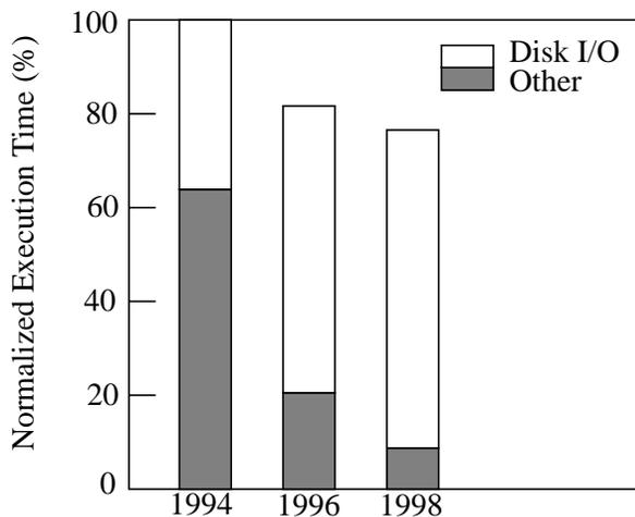
**Figure 1: Database Execution Time Profile on Next-Generation Machines.** This figure is taken from [Rosenblum95] and shows execution time of a database workload (Sybase SQL server running the TPC-B benchmark) on three machine models. The time is normalized to the speed of the 1994 model. Without reliable memory, disk I/Os will be the first-order bottleneck to higher performance.
