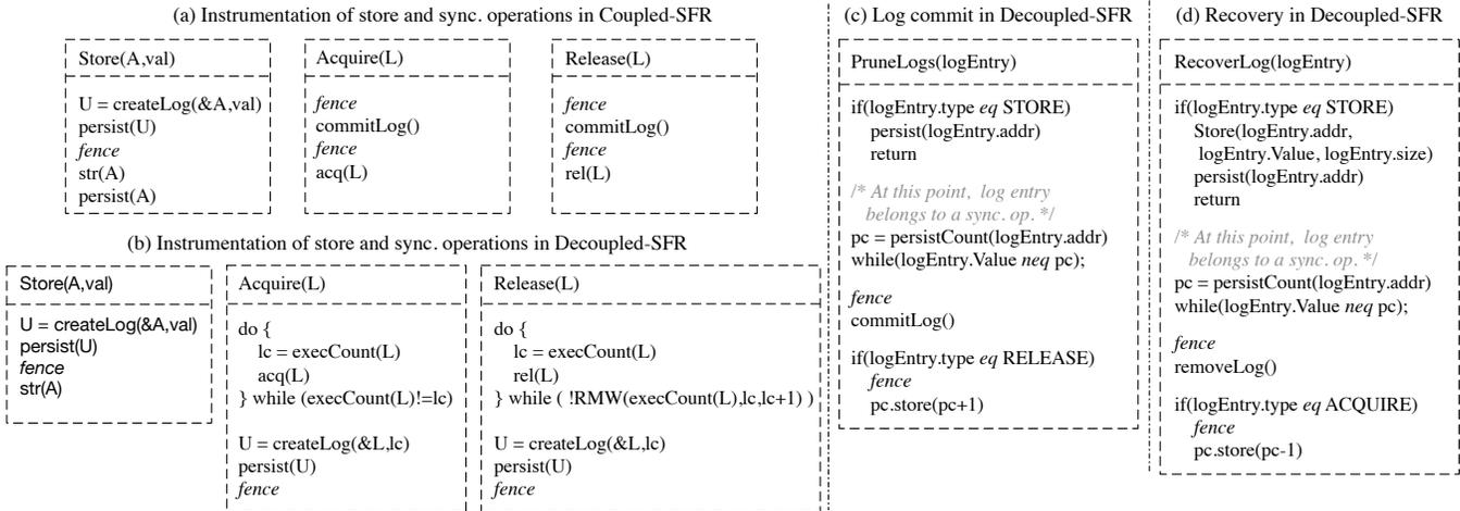
**Figure 4.** (a) Instrumentation for store and synchronization operations in Coupled-SFR design. (b) Instrumentation for store and synchronization operations in Decoupled-SFR design. Acquire (acq) and release (rel) operations are atomic loads and atomic stores to the synchronization variable L. (c) Pseudo-code for log commit operation by pruner threads in Decoupled-SFR design. (d) Pseudo-code for recovery operation at failure in Decoupled-SFR design.
