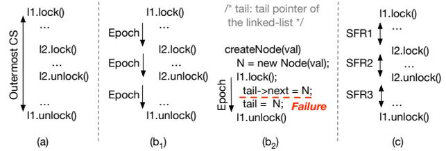
**Figure 1.** (a) Failure atomicity for outermost critical sections in ATLAS, (b<sub>1</sub>) Epoch ordering in ARP, (b<sub>2</sub>) Unclear failure atomicity semantics in ARP resulting in partial updates in PM, and (c) Our proposal: failure atomicity for SFRs.
