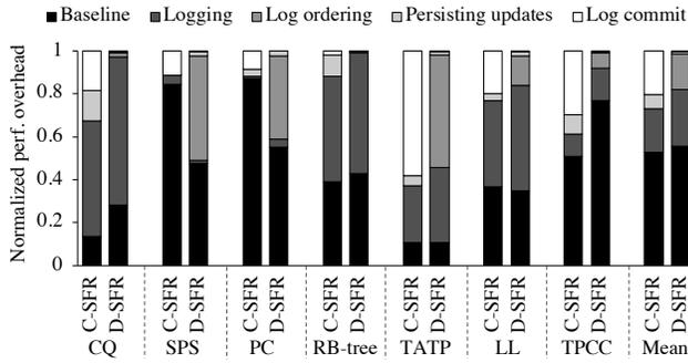
**Figure 6.** Distribution of logging overhead in Coupled-SFR and Decoupled-SFR designs.
