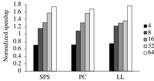
**Figure 8.** Sensitivity study showing speedup of Decoupled-SFR normalized to Coupled-SFR with increasing number of stores per SFR.
