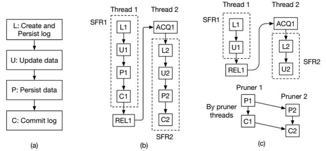
**Figure 2.** (a) Steps in undo logging mechanism, (b) Undo log ordering in Coupled-SFR when SFRs are durability-ordered, and (c) Undo log ordering in Decoupled-SFR when SFRs are durability-ordered.
