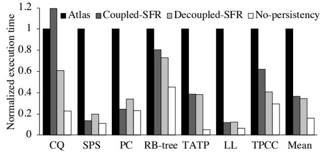
**Figure 5.** Execution time of Coupled-SFR and Decoupled-SFR designs normalized to ATLAS. No-persistence design, with no durability guarantees, shows an upper bound on performance.
