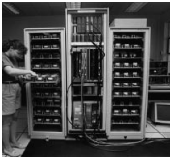
Figure 3: The physical packaging of the RAID-II File Server. Two outer racks contain 144 disks and their power supplies. The center rack contains three chassis: the top chassis holds VME disk controller boards; the center chassis contains XBUS controller boards and HIPPI interface boards, and the bottom VME chassis contains the Sun4/280 workstation.
