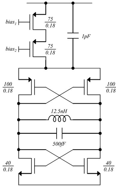
Figure 3. CMOS LC oscillator with noise reduction enhancements
