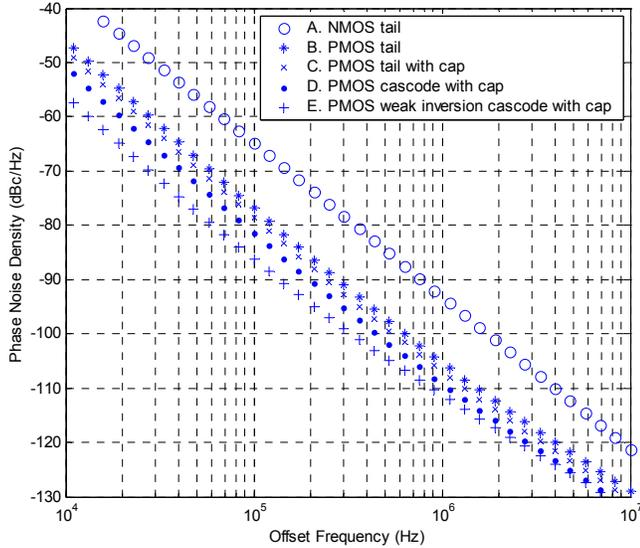
Figure 4. Phase noise spectral density results for each topology
