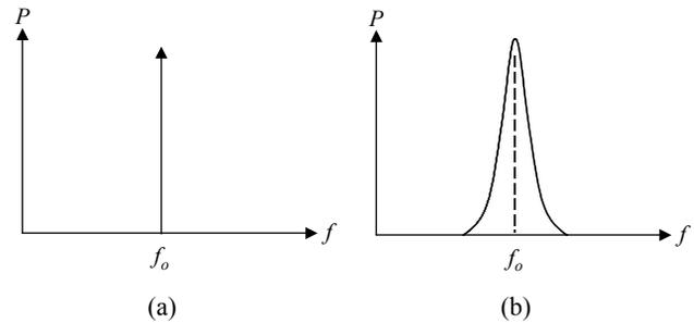
Figure 1. Output spectrum (a) ideal (b) with phase noise
