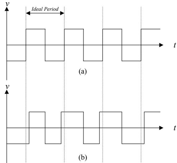
Figure 2. Time domain output (a) ideal (b) with jitter
