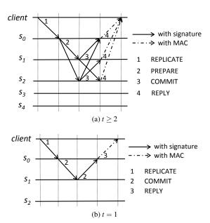
Figure 2: XPaxos common-case message patterns (a) for the general case when  $t \ge 2$  and (b) for the special case of t = 1. The synchronous groups are  $(s_0, s_1, s_2)$ and  $(s_0, s_1)$ , respectively.
