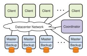
**Figure 1:** RAMCloud cluster architecture. Each storage server contains a master and a backup. A central coordinator manages the server pool and tablet configuration. Client applications run on separate machines and access RAMCloud using a client library that makes remote procedure calls.
