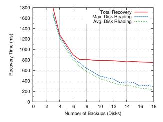
**Figure 7:** Recovery time as a function of the number of disks, with a single recovery master, one 600 MB partition with 1,024 byte objects, and each disk on a separate machine. "Avg. Disk Reading" measures the average elapsed time (across all disks) to read backup data during recovery; "Max. Disk Reading" graphs the longest time for any disk in the cluster. Once 6-8 disks are available recovery time is limited by the network of the recovery master
