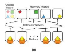
Figure 3: (a) Disk bandwidth is a recovery bottleneck if each master's data is mirrored on a small number of backup machines. (b) Scattering log segments across many backups removes the disk bottleneck, but recovering all data on one recovery master is limited by the network interface and CPU of that machine. (c) Fast recovery is achieved by partitioning the data of the crashed master and recovering each partition on a separate recovery master.
