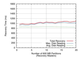
**Figure 8:** Recovery performance under proportional scaling (one recovery master and 6 backups for each 600 MB partition of data to recover). Each recovery master shared a host with 2 backups, and each point is an average of 5 runs (Figure 11 shows the variance between runs). A horizontal line would indicate perfect scalability. Recovery time is limited by disk bandwidth.
