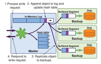
**Figure 2:** When a master receives a write request, it updates its in-memory log and forwards the new data to several backups, which buffer the data in their memory. The data is eventually written to disk or flash in large batches. Backups must use an auxiliary power source to ensure that buffers can be written to stable storage after a power failure.
