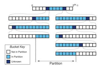
**Figure 5:** A tablet profile consists of a hierarchical collection of bucket arrays; buckets are subdivided dynamically when their counts become large. The tree structure creates (bounded) uncertainty when assigning partition boundaries, since counts in ancestor buckets may represent objects either before or after the boundary.
