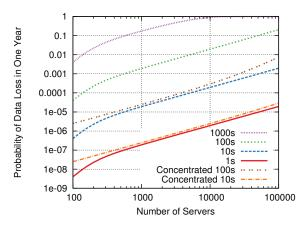
**Figure 12:** Probability of data loss in one year as a function of cluster size, assuming 8,000 segments per master, two disk replicas for each DRAM copy, and two crashes per year per server with a Poisson arrival distribution. Different lines represent different recovery times. Lines labeled "Concentrated" assume that segments are concentrated instead of scattered: each master picks 2 backups at random and replicates all of its segments on each of those backups.
