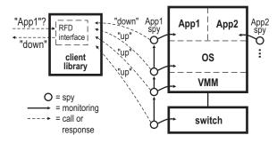
**Figure 1**—Architecture of Falcon. The application spy provides accurate information about whether the application is up; this spy is the only one that can observe that the application is working. The next spy down provides accurate information not only about its layer but also about whether the application spy is up; more generally, lower-level spies monitor higher-level ones.
