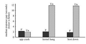
**Figure 12**—Median response gap (unavailability) of ZooKeeper [31] with Falcon-NoKill (F) and unmodified (Un) under injected failures at the leader. In unmodified ZooKeeper, followers quickly detect application crashes but not kernel- or host/VMM-level crashes. Under the latter types, Falcon reduces median ZooKeeper unavailability by roughly a factor of 6. In all cases, unavailability is several seconds on top of detection time because of ZooKeeper's recovery time.
