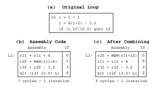
Figure 6: Example of operation combining.
