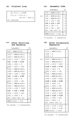
Figure 3: Example of accumulator variable expansion.
