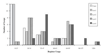
Figure 15: Register usage distribution of non-DOALL loops only for an issue-8 superscalar/VLIW processor.
