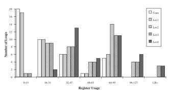
Figure 11: Register usage distribution for an issue-8 superscalar/VLIW processor.
