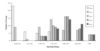
Figure 8: Speedup distribution for an issue-2 superscalar/VLIW processor.
