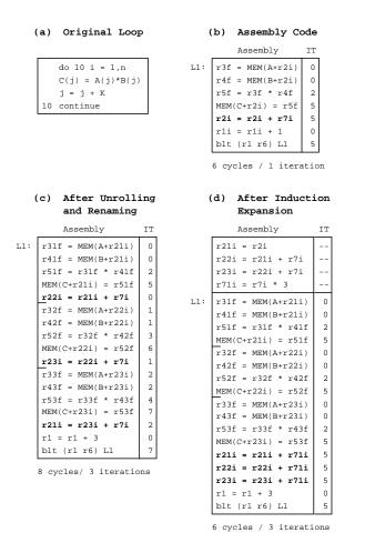
Figure 5: Example of induction variable expansion.
