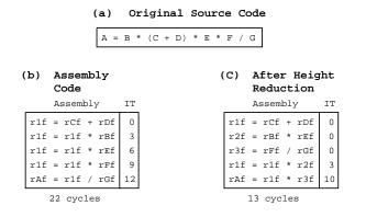
Figure 7: Example of tree height reduction.
