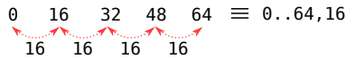
Fig. 8. Example of a monotonically increasing sequence that grows by a fixed value.
