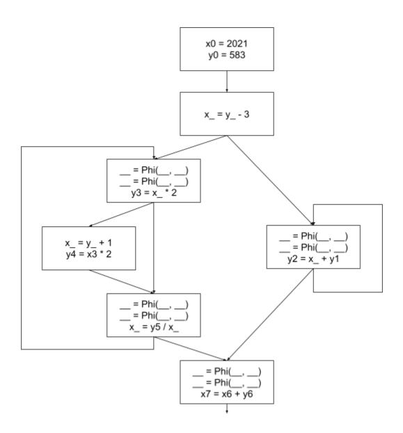
10) You want to apply Loop Invariant Code Motion (LICM) to the CFG below. Insert the following instructions I1-I4 into BB1-BB4 with a maximum of 1 instruction added to each BB (i.e., one instruction in BB1, one in BB2, etc.) so that LICM can hoist as many instructions as possible. Just mark on the CFG below where the instructions should be placed and indicate whether they can be hoisted to the preheader. For those instructions that could not be hoisted, specify a reason. (15 pts)
