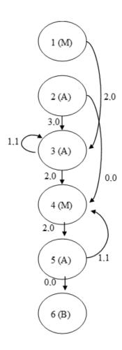
Processor model 2 fully pipelined function units 1 ALU, 1 MEM
