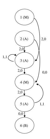
Processor model 2 fully pipelined function units 1 ALU, 1 MEM
