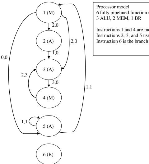
6 fully pipelined function units
