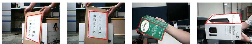
**Fig. 3.** Tracking failures when boundary correction (line features) is disabled. The failures are caused primarily by either accumulated feature position error or accumulated parameter estimation error.
