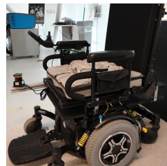
Fig. 1. We calibrate and evaluate our dynamic model with a powered wheelchair, and show that it allows very fast (over 10^5 times faster than real-time) and reliable long-term prediction of vehicle velocities. The vehicle ( \sim 120 kg) has two drive wheels powered by two electric motors, four castor wheels, and a joystick input device.
