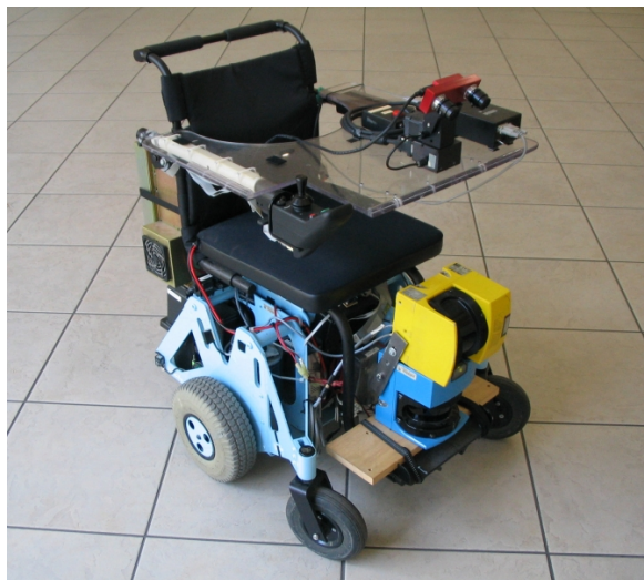
Figure 1.1: The wheelchair robot used as the experimental platform in this work. The robot has a stereo camera and one horizontal and one vertical laser range-finder.
