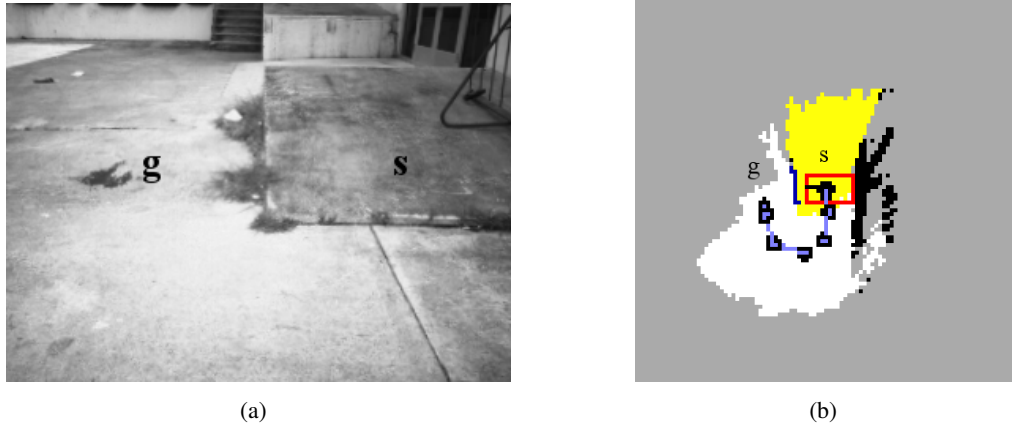
Figure 2.2: Path planning using the safety map. (a) Image from the stereo camera on the Intelligent Wheelchair showing an environment with an upward ramp and the resulting drop-off edge. (b) The safety map of the environment showing the robot (in red) and a planned path (in blue-black) from start, s , to goal, g . The start and end points are also shown in the stereo camera image. The safety map coloring scheme is as follows: “Level” regions are in white; “Non-ground” regions in black; “Inclined” regions are in yellow (representing the upward ramp in this case); “Unknown” regions are in gray; and “Drop-off Edge” cells on the ramp are in blue. The planning algorithm treats these blue cells (next to the actual drop-off boundary) as unsafe and plans a path around them even though the goal is directly ahead of the robot.
