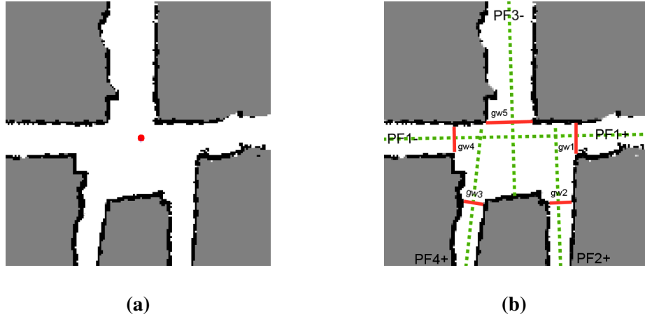
Figure 2.3: A local metrical map and its local topology. (a) A grid map of a small scale environment constructed using laser range-finders. The white areas represent free space, black areas represent obstacles, and grey areas represent unexplored space. We call such a small scale map a local metrical map. The robot is shown as a circle in its center. (b) A pictorial representation of the local topology of the place described by the local metrical map. The dashed green segments represent path fragments (PF1, PF2, etc) that pass through or terminate in the place whereas the solid red segments (gw1, gw2, etc) are gateways into and out of the place [Beeson et al., 2005].
