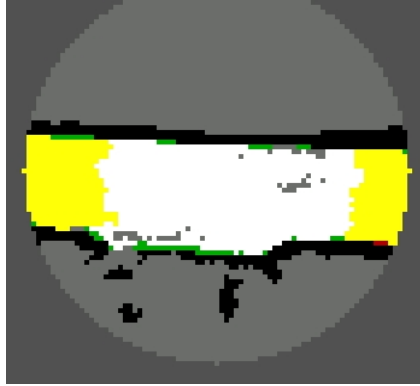
Figure 8.10: Safety map of the BIORAMP environment showing false positive cells in green and false negative cells in red. Most of these cells occur on the boundary between safe and unsafe regions.
