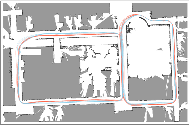
Figure 3: The test environment used for evaluation, showing trajectories generated by MPEPC (blue) and SA-MPEPC (orange). All trajectories follow a figure-of-eight pattern, CW around the left loop and CCW around the right loop. (This figure is best viewed magnified and in color.)
