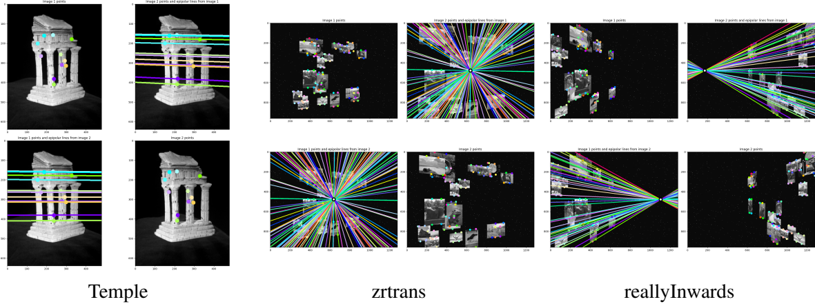
Figure 1: Epipolar lines for some of the datasets. The Epipoles are marked in little white circles. Best seen by zooming in.
