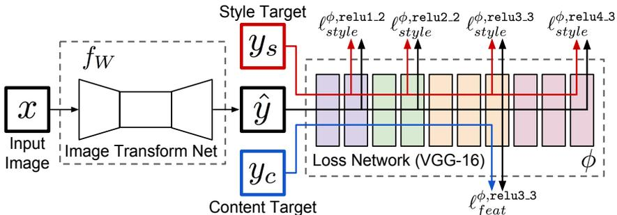
**Fig. 2.** System overview. We train an *image transformation network* to transform input images into output images. We use a *loss network* pretrained for image classification to define *perceptual loss functions* that measure perceptual differences in content and style between images. The loss network remains fixed during the training process.
