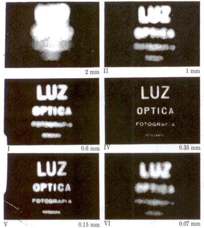
Fig. 5.96 The pinhole camera. Note the variation in image clarity as the hole diameter decreases. [Photos courtesy Dr. N. Joel, UNESCO.]
